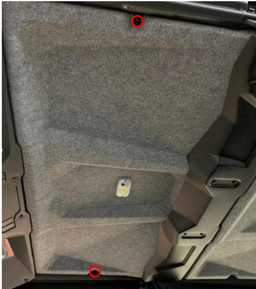
Figure 6: Remove the screws from the sides of the front roof liner.
