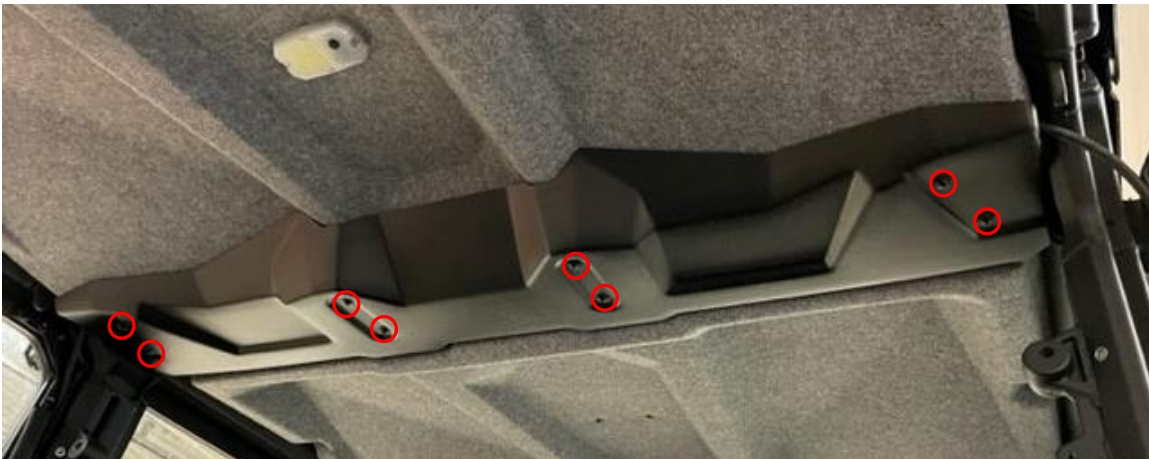
Figure 4: Remove the center roof liner support. Defender MAX models only.
