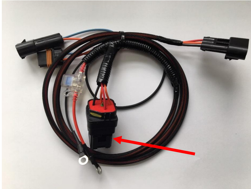
Figure 2: Chassis harness ignition relay
