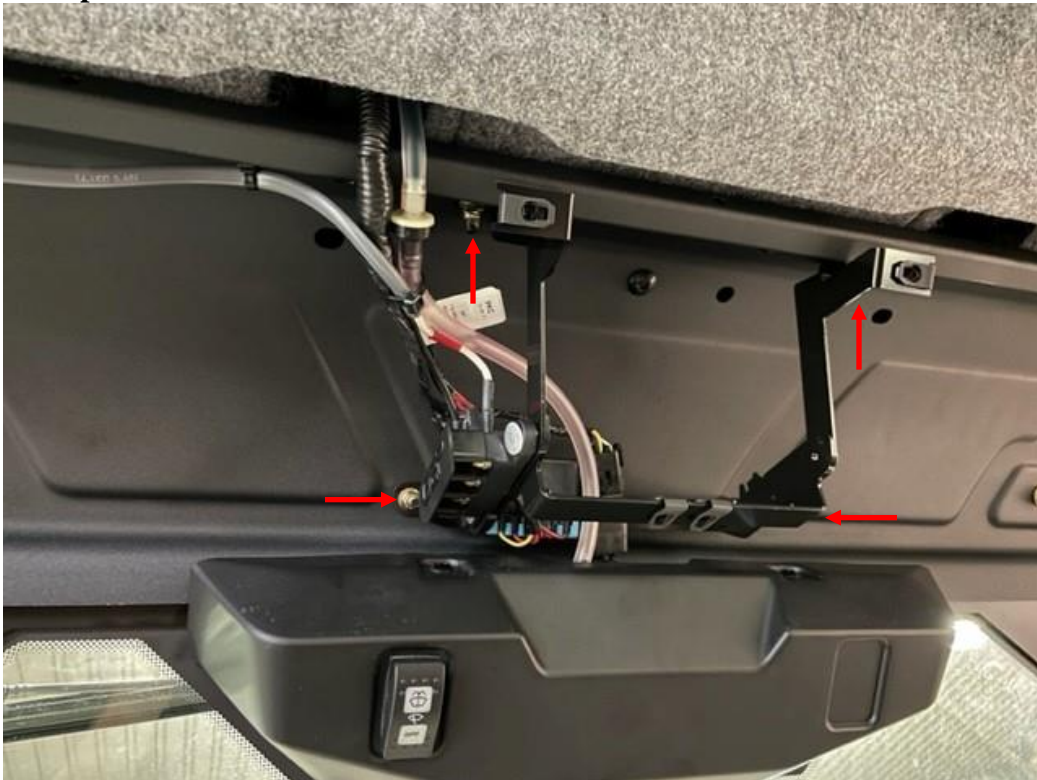
Figure 10: Remove the center roof liner bracket.
