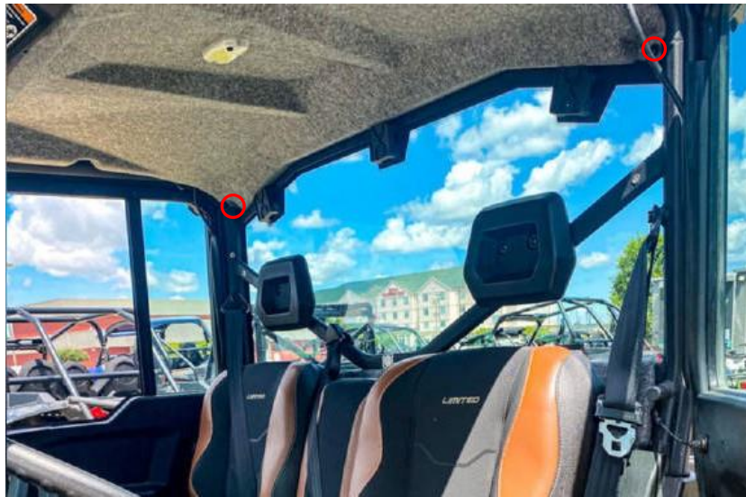
Figure 5: Remove the bolts from the rear of the liner. Defender single-row models only.
