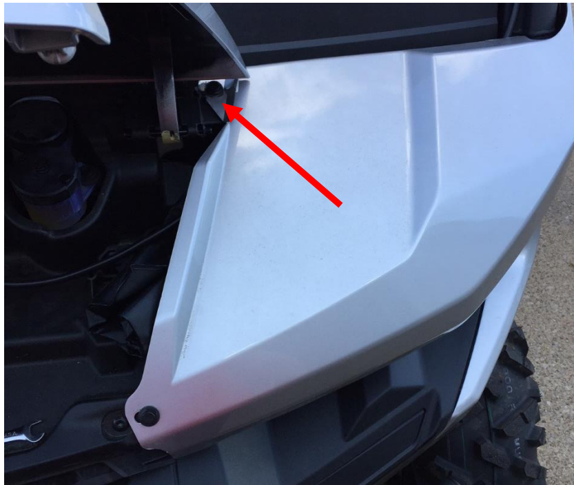
Figure 26: Remove the plastic rivet to run the chassis harness under the panel.
