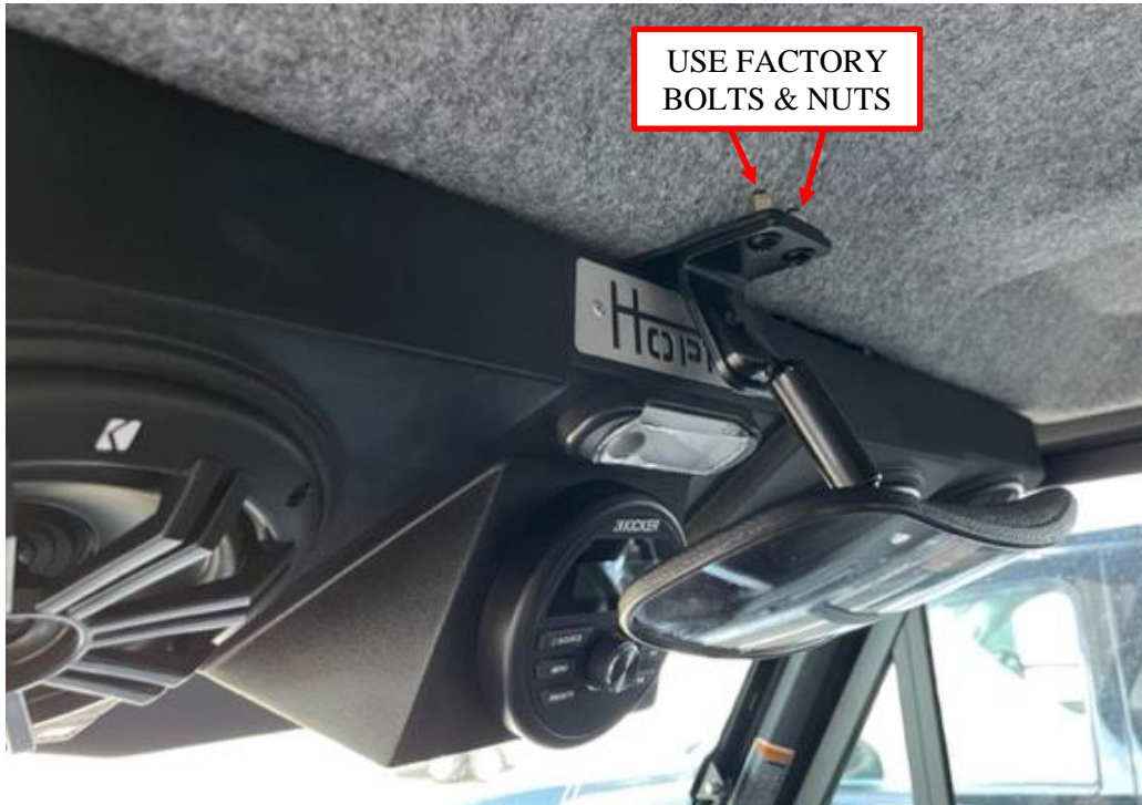
Figure 23: Mount the rearview mirror on the bracket.
