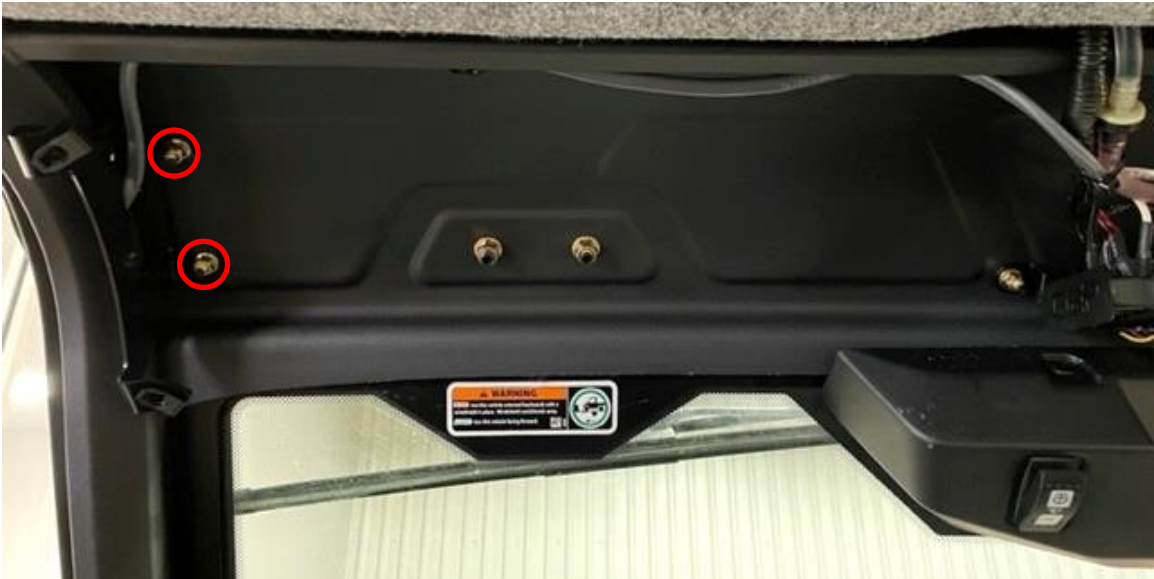
Figure 9: Remove the roof liner brackets. Driver side shown. (Passenger side similar)
