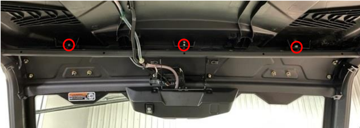
Figure 8: Remove 3 bolts to loosen the roof.
