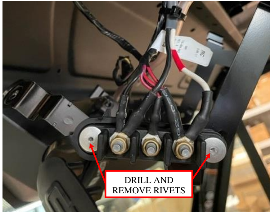
Figure 11: Drill and remove rivets to remove terminal block.
