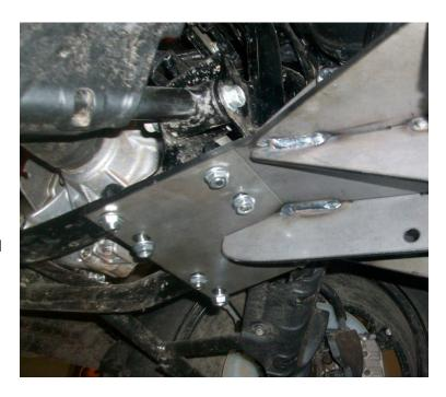
Attach the lower under portion to the frame tubes as shown using the 4 - u-bolts, 8 - washers and nylock nuts.
