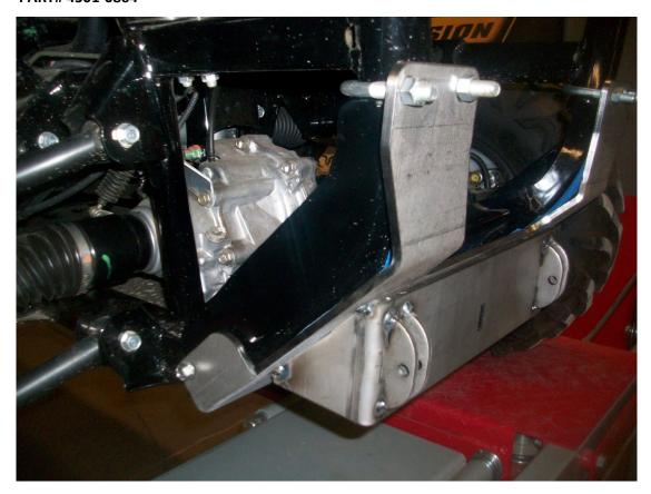
Remove the front lower bumper plate bolts on each side of the machine.
