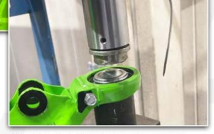
NOW SET THE BALL JOINT INTO THE NEW ARM AND PRESS IT INTO PLACE USING THE SAME SOCKET AS BEFORE.
