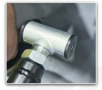
INSTALL THE LOWER ARMS AT THE FRAME USING THE FACTORY (17MM) NUTS AND BOLTS. LOOSELY TIGHTEN AT THIS TIME.
