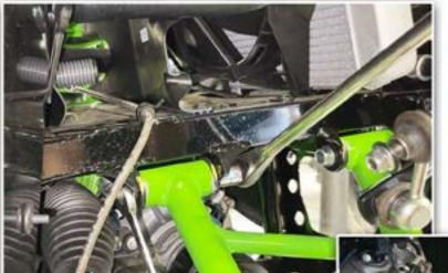
NOW REMOVE THE BOLTS AND NUTS HOLDING THE UPPER ARM TO THE FRAME. (17MM)
