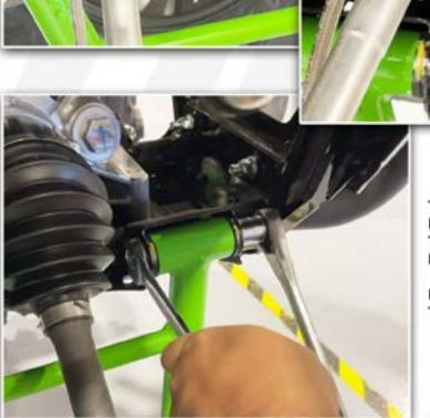
THEN, REMOVE THE (17MM) NUTS AND BOLTS HOLDING THE LOWER A-ARM TO THE FRAME.
