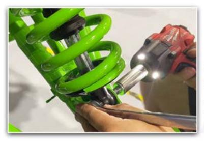
NEXT, REMOVE THE BOLT AND NUT FROM THE SHOCK TAB. (17MM)
