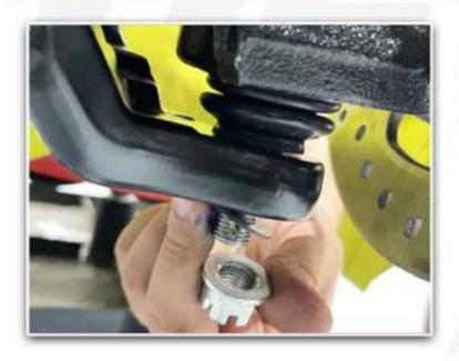
NOW INSTALL THE BALL JOINT ON THE KNUCKLE INTO THE LOWER ARM USING THE FACTORY (19MM) NUT AND WASHER.
