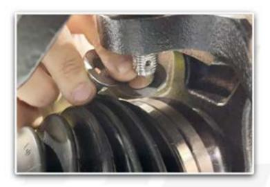
INSTALL THE SWAY BAR USING THE FACTORY (14MM) WASHER AND NUT.
