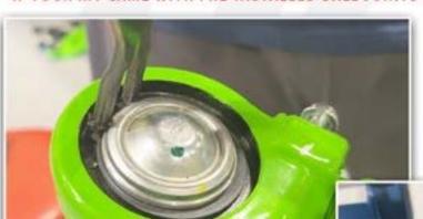
FIRST REMOVE THE RETAINING CLIP. YOU WILL NEED A PRESS AND A SOCKET THAT IS THE SAME DIMENSIONS AS THE BALL JOINT TO PRESS THE BALL JOINT OUT.
