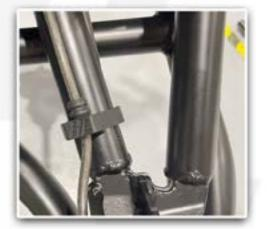
ATTACH THE SHOCK TO THE ARM USING THE FACTORY (17MM) NUT AND BOLT. LOOSELY TIGHTEN.
