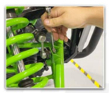
REMOVE THE FACTORY SWAY BAR NUT. (14MM) MAY HAVE TO TAP THE SWAY BAR LOOSE FROM THE TAB WITH HAMMER.
